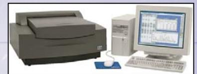
Fig.11. Image-plate scanner
