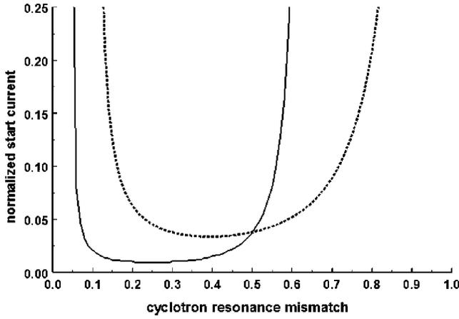
FIG. 1. Normalized start current as the function of the cyclotron resonance detuning  $\Delta$  for two values of the normalized interaction length,  $s_{\text{out}}=10$  (dotted line) and  $s_{\text{out}}=15$  (solid line).
