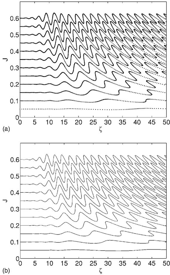
FIG. 8. Varying frequency mismatch. (a) Numerically and (b) analytically [Eqs. (20) and (21)] obtained Poincaré surface of section  $\Sigma^{\theta_0=0}$ . Parameter set:  $F=0.01$ ,  $\Delta=0.5$ ,  $\mu=15$ ,  $n=2$ ,  $\delta^{(1)}=-0.05$ .
