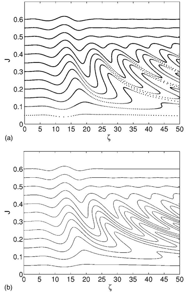
FIG. 1. (a) Numerically and (b) analytically [Eqs. (20) and (21)] obtained Poincaré surface of section  $\Sigma^{\theta=0}$ . Parameter set:  $F=0.01$ ,  $\Delta=0.5$ ,  $\mu=15$ ,  $n=1$ .
