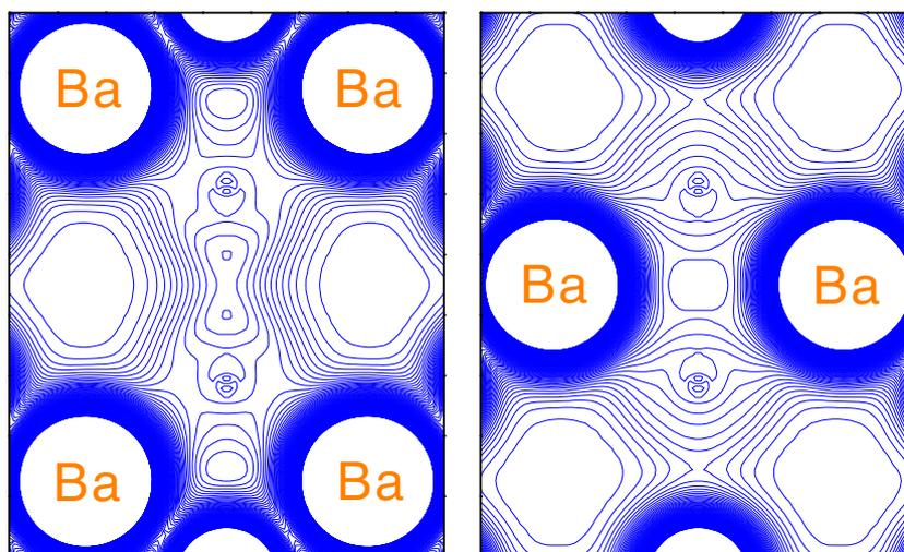
**Figure 8.** Charge density map of a BaF<sub>2</sub> crystal with the periodic M centre from the (1 1 0) (left) and (1  $\bar{1}$  0) (right) side view. Isodensity curves are drawn from 0 to 0.1  $e/\text{bohr}^3$  with an increment of 0.001  $e/\text{bohr}^3$ .
