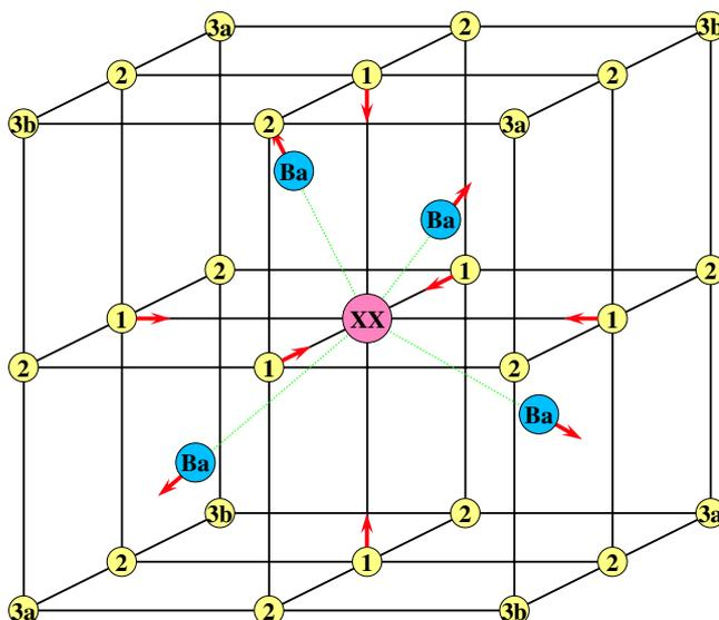
**Figure 5.** A view of the F-centre nearest-neighbour geometry in  $\text{BaF}_2$  with the indication of relaxation shifts. The position of the colour centre is indicated by XX. The fluorines are labelled 1 in the first shell, 2 in the second shell and 3a and 3b in the third shell.
