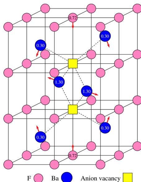
**Figure 7.** A view of the M-centre nearest-neighbour geometry in BaF<sub>2</sub> with indication of relaxation shifts. The positions of the anion vacancies are indicated by two squares. The directions of atomic displacements are shown with arrows; the values are given as a percentage of the lattice constant.
