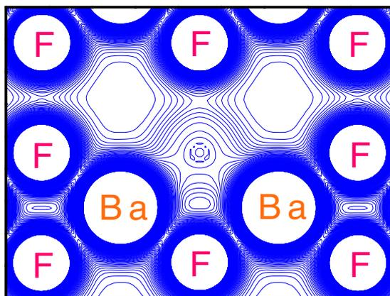
**Figure 4.** Charge density map of BaF<sub>2</sub> with F centre from the (110) side view. Isodensity curves are drawn from 0 to 0.1  $e/\text{bohr}^3$  with an increment of 0.001  $e/\text{bohr}^3$ .
