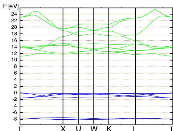
Figure 1. Electronic band structure of BaF<sub>2</sub> bulk calculated by means of the hybrid B3PW method.
