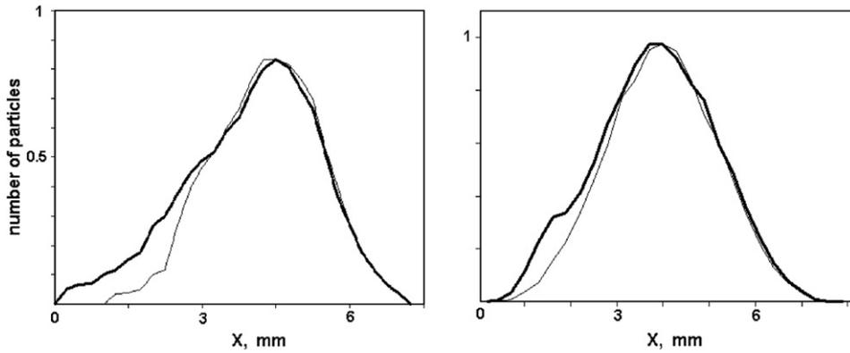
Fig. 4. The experimentally measured beam profiles (at the left) and result of simulation (on the right) in 0.5 m downstream of crystal. Thick lines correspond to penetration of beam in bent part of a crystal strip. Thin lines correspond to section, where the crystal was straight.
