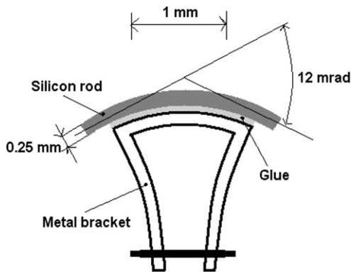
Fig. 5. Another-type of bent crystal. A bending angle of 12 mrad is obtained, owing to the pressure of a metallic microbracket.
