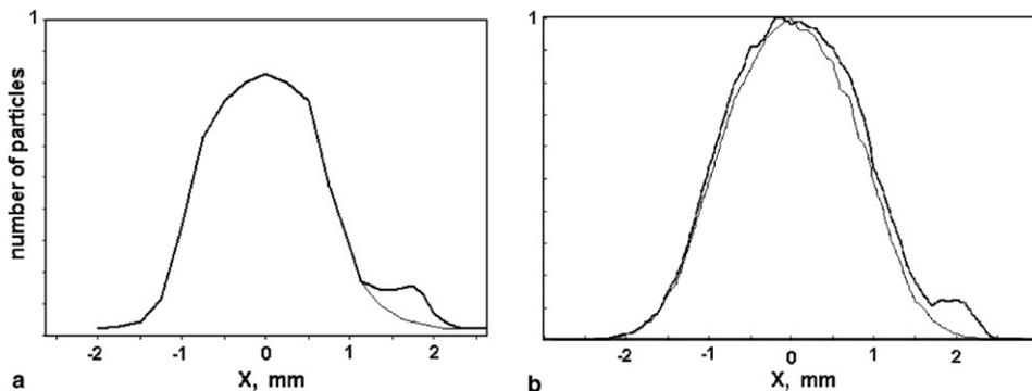
Fig. 6. The experimentally measured beam profiles (a) and result of simulation (b) in 0.17 m downstream of 12 mrad bent crystal. Thick lines correspond to penetration of beam in oriented crystal (effect of crystal channeling is seen on the right side of plots). Thin lines correspond to disoriented crystal. In experimental plots 10% level of statistical fluctuations of emulsion analysis data are not shown.
