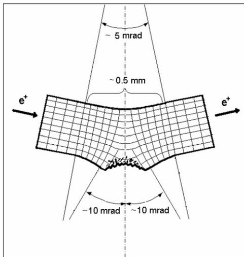
Fig. 2. Scheme of the crystal deformation due to a mechanical scratch.
