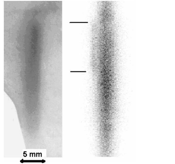
Fig. 3. The image of collimated beam scattered on the crystal measured with emulsion layer at 0.5 m downstream (at the left) and result of Monte Carlo simulation (at the right).
