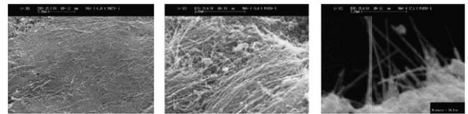
Fig. 7a. SEM images of CNTs synthesized at INFN – LNF.
