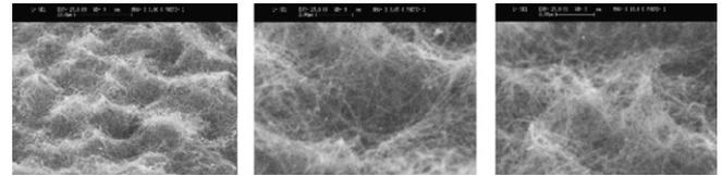
Fig. 7b. A carpet of CNTs synthesized at INFN – LNF with an arc-discharge setup.
