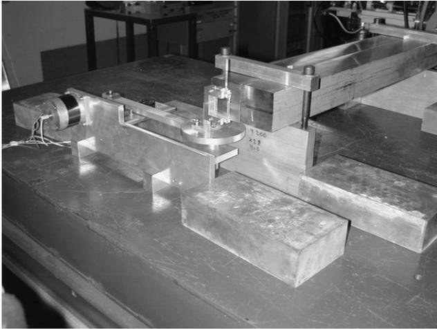
Fig. 1. Goniometer for crystal sample rotation (30  $\mu$ rad step) in front view and steel collimator in back view.
