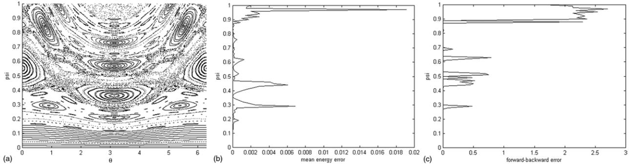
**Figure 1.** (a) The phase portrait of the HJ-tokamak corresponding to  $q(0) = 1$  and  $\varepsilon = 6/(4\pi^2) \approx 0.152$ ; (b) the mean energy errors of the orbit drawn in (a); (c) the forward–backward errors of the orbits drawn in (a).
