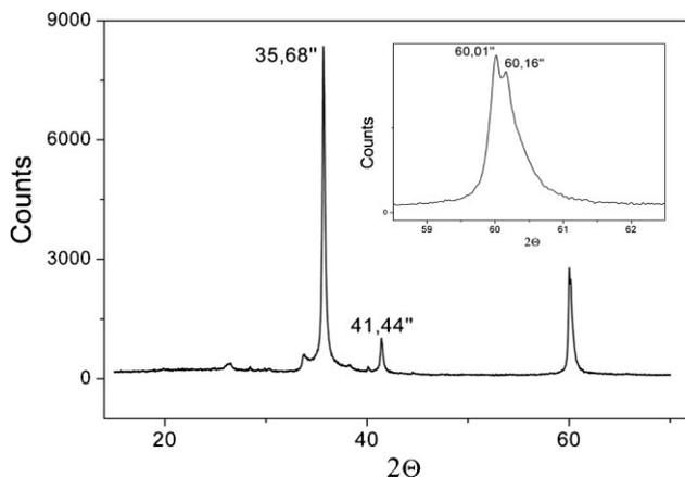
**Figure 1** XRD pattern of as-obtained SiC nanowires.
