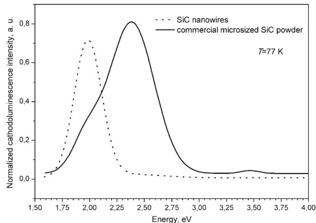
**Figure 2** The difference in the cathodoluminescence from the bulk 3C-SiC and obtained silicon carbide nanowires. Intensities are normalized for the purpose of comparison.
