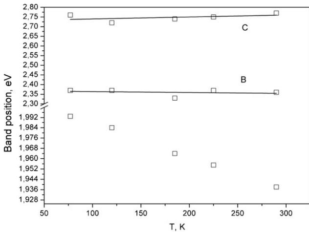
**Figure 4** Peak positions of luminescence bands versus temperature (SiC nanowires). Solid lines represent linear fit for bands B and C.
