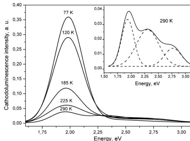
**Figure 3** CL from obtained SiC nanowires at elevating temperatures. The inset illustrates the spectrum at 290 K in which three Gaussian components are shown as dashed lines.
