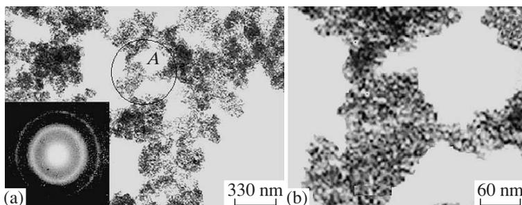
**Fig. 2.** TEM images of dest-5YSZ nanopowders: (a) combined with an inserted MD, (b) magnified image of area A (in circle).
