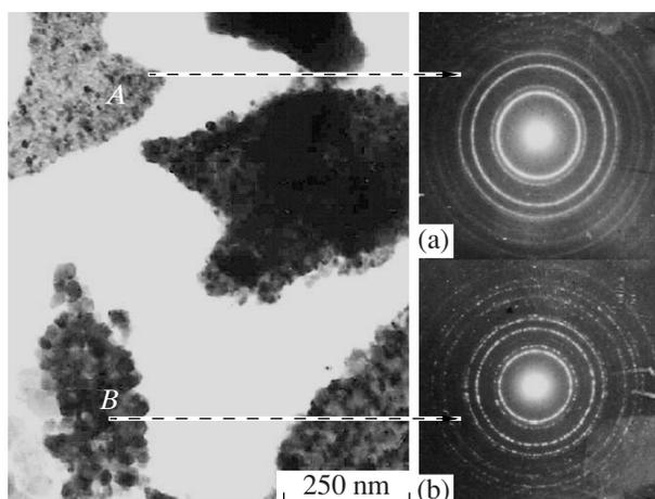
**Fig. 1.** TEM images illustrating morphological and structural non-homogeneity of nanopowders obtained by glycine method, and microdiffraction patterns (a, b) corresponding to A and B areas.
