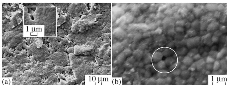
**Fig. 4.** Surface topography of ceramics produced from dest-0XYZ nanopowders in square-magnified part (a); from dest-5YSZ (b).
