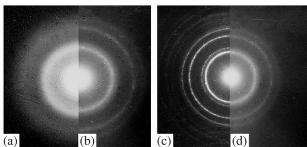
**Fig. 3.** Microdiffraction patterns from dest-0YSZ (a), dest-5YSZ (b), glc-5YSZ (c), and dest-5YSZ (d) nanopowders.
