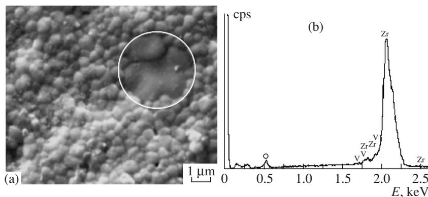
**Fig. 5.** Ceramic surface of glc-5YSZ powders after compacting and sintering at 1500°C in vacuum (a); the energy dispersive spectrum from the area inside circle (b).
