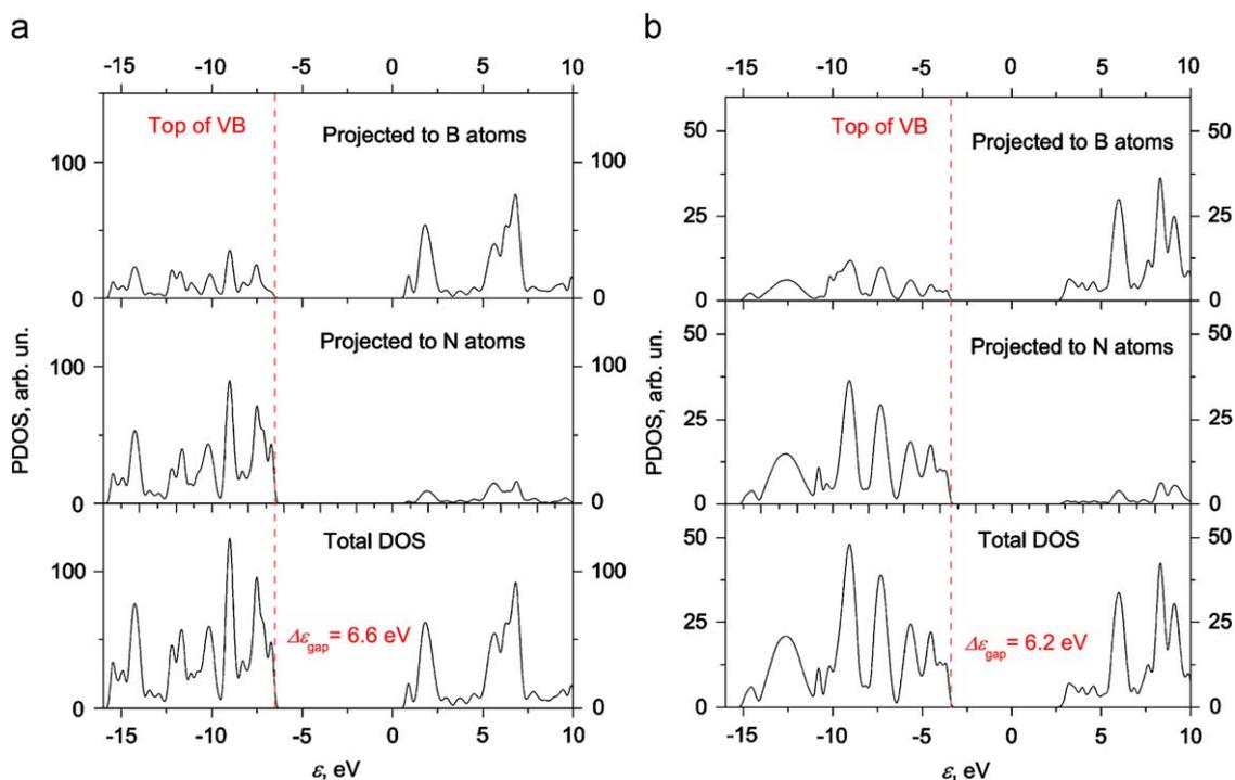
**Fig. 4.** Total and projected densities of one-electron states (DOSs) for (a) *h*-BN (Fig. 1(a)) and (b) *c*-BN (Fig. 1(b)) bulk calculated using hybrid B3PW Hamiltonian [43]. Details of DOSs are described inside the plots; moreover, values of  $\Delta\epsilon_{\text{gap}}$  are also presented in Table 1. (For interpretation of the references to colour in this figure legend, the reader is referred to the web version of this article.)
