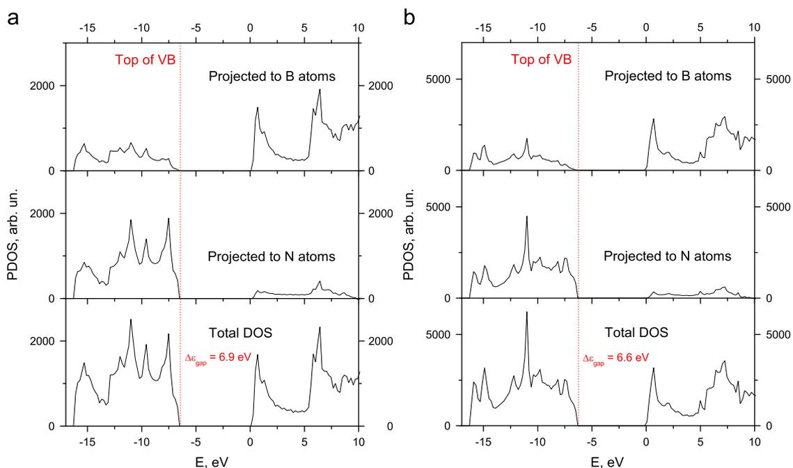
**Fig. 5.** The total and projected densities of one-electron states (DOSs) for BN NTs: (a) 5 nm armchair-type (36,36) (Fig. 2(a)) and (b) 5 nm zigzag-type (64,0) (Fig. 2(b)). For details, see explanations given in Fig. 4. (For interpretation of the references to colour in this figure legend, the reader is referred to the web version of this article.)
