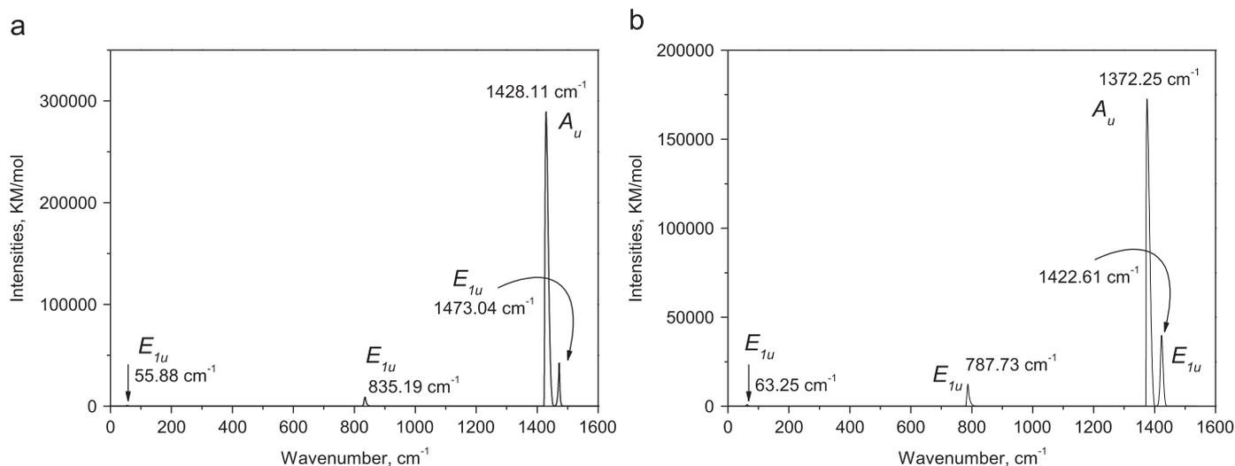
Fig. 6. Frequencies and intensities of IR active TO phonon mode for *ac*-BN NT calculated using B3PW (a) and PWGGA (b) methods.
