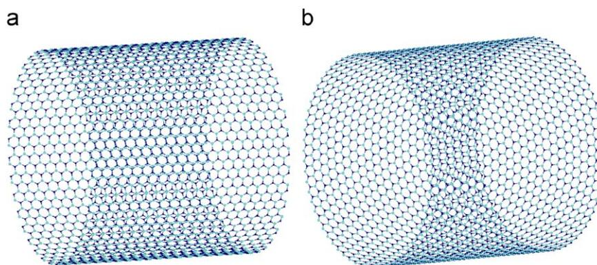
**Fig. 2.** Fragments of 5-nm-thick 1D BN nanotubes: (a) armchair-type chirality (rod symmetry  $Pn/m$ )-(36,36) unit cell with periodicity 2.55 Å and (b) zigzag-type chirality (rod symmetry  $Pnmm$ )-(64,0) unit cell with periodicity 4.45 Å. Light turquoise balls correspond to B atoms and N atoms are shown by dark blue. (For interpretation of the references to colour in this figure legend, the reader is referred to the web version of this article.)
