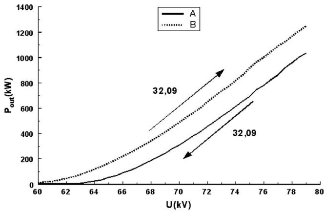
FIG. 5. Output power as a function of voltage in cavities *A* (solid line) and *B* (dotted line). Calculations were carried out from 60 to 79 kV and from 79 to 60 kV. No parasitic modes are excited, no hysteresis is seen.
