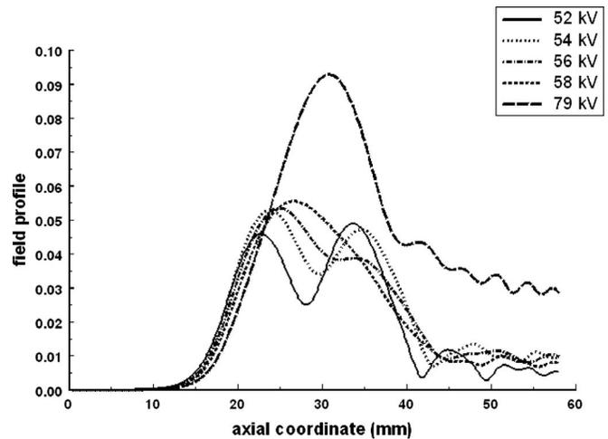
FIG. 4. Axial profile of the operating mode at several voltages. The field profile between 52 and 58 kV changes from two maxima to one maximum. Between 58 and 79 kV just the magnitude of the field profile is rising.
