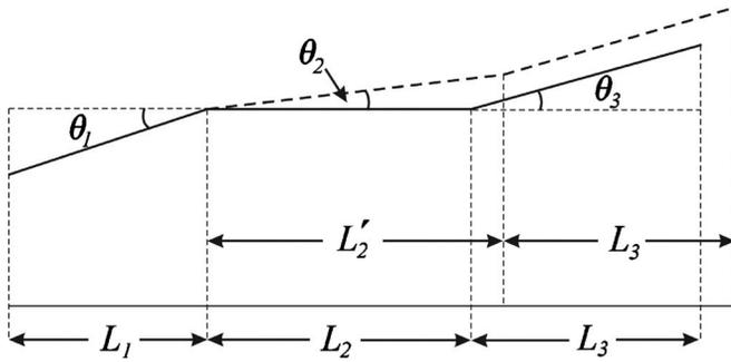
FIG. 1. Profiles of a standard resonator with the constant radius of its central part (solid lines) and that of a slightly uptapered resonator (dashed lines).
