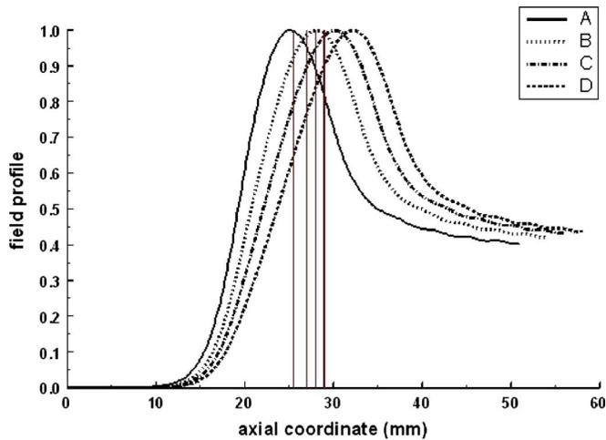
FIG. 2. (Color online) Axial profiles of the operating mode field in several resonators. Vertical lines mark the middle point of the cavity (25.5 mm for *A*, 27 mm for *B*, 28 mm for *C*, and 29 mm for *D*). Note that tapering shifts the maximum of the field profile toward the output end.
