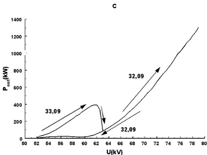
FIG. 6. Output power as a function of voltage. Calculations were carried out from 50 to 79 kV and from 79 to 50 kV. At low voltages, the parasitic  $TE_{33,09}$  mode is excited. At 63 kV it is replaced by the operating  $TE_{32,09}$  mode. Due to hysteresis when decreasing the voltage the operating mode survives until 52 kV. A clear hysteresis loop is seen.
