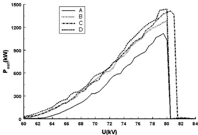
FIG. 3. Dependence of the output power on the beam voltage.
