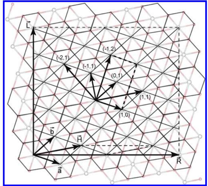
**Figure 1.** Chiral  $\mathbf{R}$  (4,2), translation  $\mathbf{L}$  (-4,5), helical  $\mathbf{H}$  (1,1) and special chirality vectors for hexagonal lattice.
