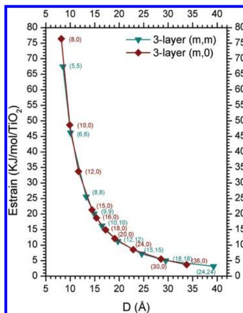
**Figure 9.** Strain energies  $E_{strain}$  vs  $D_{NT}$  for the two sets of SW TiO<sub>2</sub> NTs with various chiralities.
