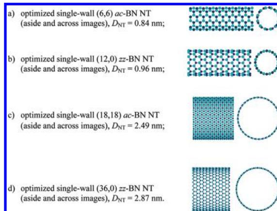
**Figure 4.** Images of hexagonal SW BN NTs with different chiralities and diameters.
