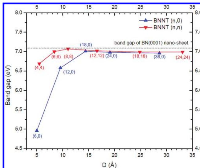
**Figure 6.** Band gaps  $\Delta\epsilon_{gap}$  vs  $D_{NT}$  for the two sets of SW BN nanotubes with various  $(n,n)$  and  $(n,0)$  chiralities.
