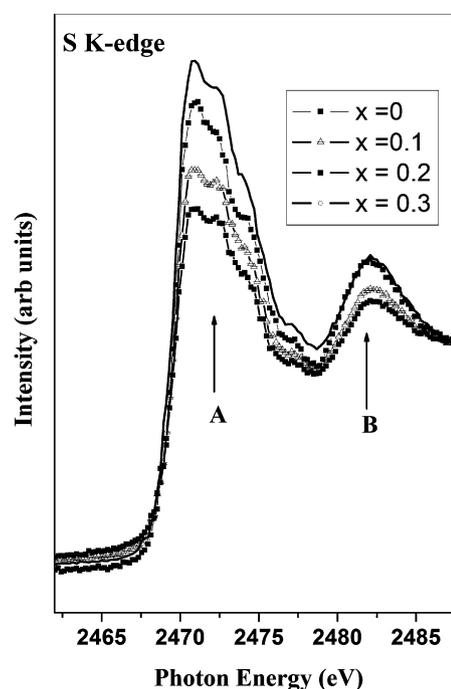
Fig. 7. XANES spectra of pure CdS and  $\text{Cd}_{1-x}\text{Co}_x\text{S}$  alloys for different Co doping concentrations ( $x=0, 0.1, 0.2$  and  $0.3$ ) [note that the oxidation state of S remains divalent with Co doping and this also indicates that the valency of Co is divalent].
