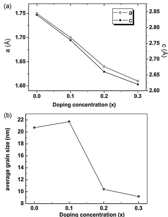
Fig. 3. (a) Lattice parameters and (b) average grain size [estimated using (002) crystal direction] of pure CdS and  $\text{Cd}_{1-x}\text{Co}_x\text{S}$  alloys for different Co doping concentrations ( $x = 0, 0.1, 0.2$  and  $0.3$ ).
