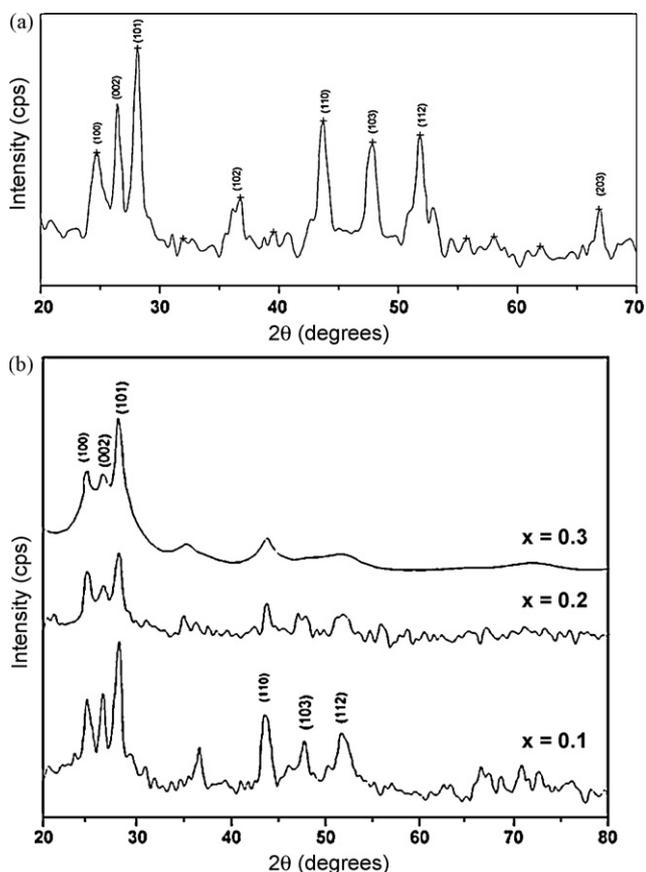
Fig. 2. X-ray diffraction spectra of (a) pure CdS and (b)  $\text{Cd}_{1-x}\text{Co}_x\text{S}$  samples.
