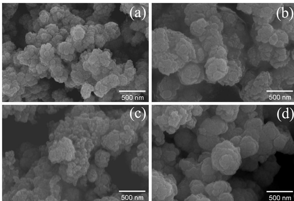
Fig. 4. FE-SEM images of (a) pure CdS, (b)  $\text{Cd}_{0.9}\text{Co}_{0.1}\text{S}$ , (c)  $\text{Cd}_{0.8}\text{Co}_{0.2}\text{S}$ , and (d)  $\text{Cd}_{0.7}\text{Co}_{0.3}\text{S}$  nanocluster alloys.
