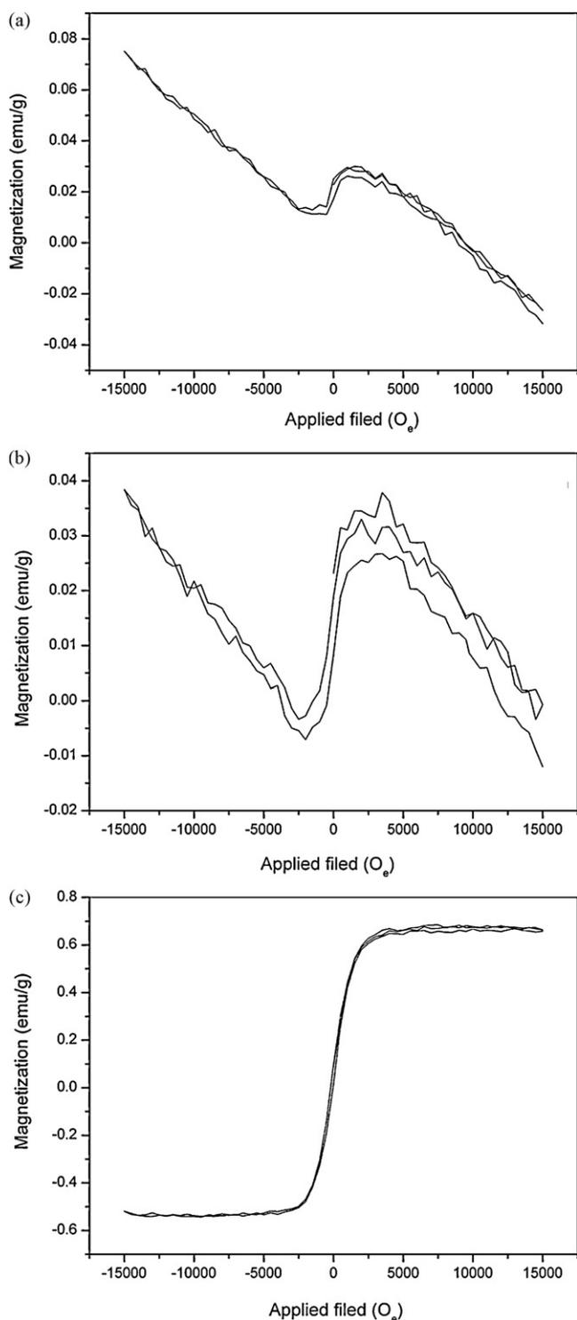
Fig. 6. Ferromagnetic behavior of a nanocluster alloys for (a)  $\text{Cd}_{0.9}\text{Co}_{0.1}\text{S}$ , (b)  $\text{Cd}_{0.8}\text{Co}_{0.2}\text{S}$ , and (c)  $\text{Cd}_{0.7}\text{Co}_{0.3}\text{S}$ .
