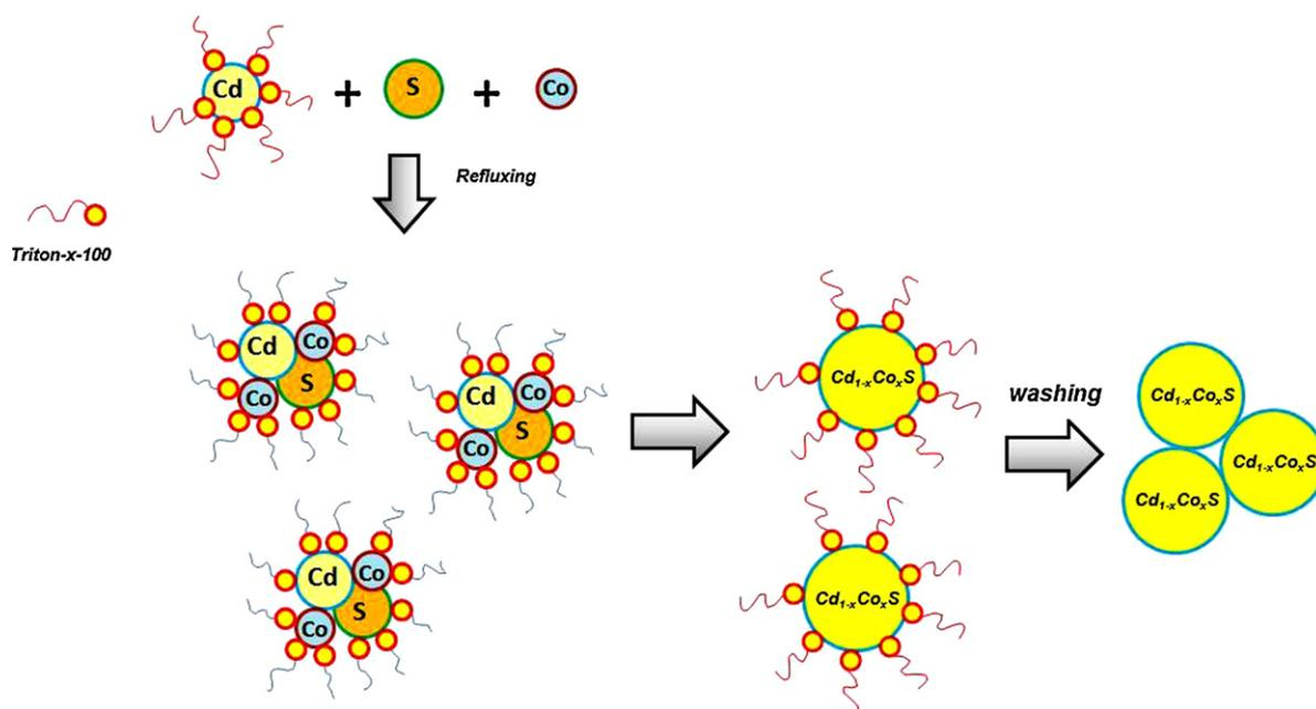
Fig. 1. Schematic growth mechanism of Cd<sub>1-x</sub>Co<sub>x</sub>S at Triton X-100 assisted medium.
