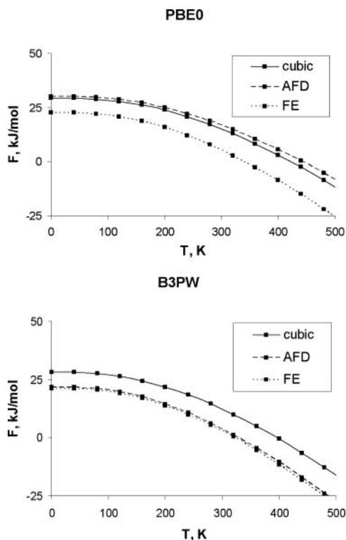
**Figure 2.** Calculated Helmholtz free energy of SrTiO<sub>3</sub> (kJ/mol).
