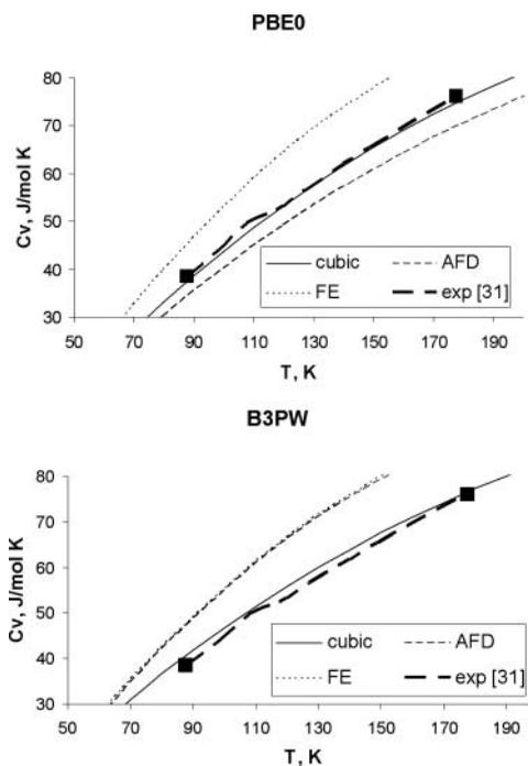
**Figure 1.** Calculated heat capacity of SrTiO<sub>3</sub> (J/mol K).
