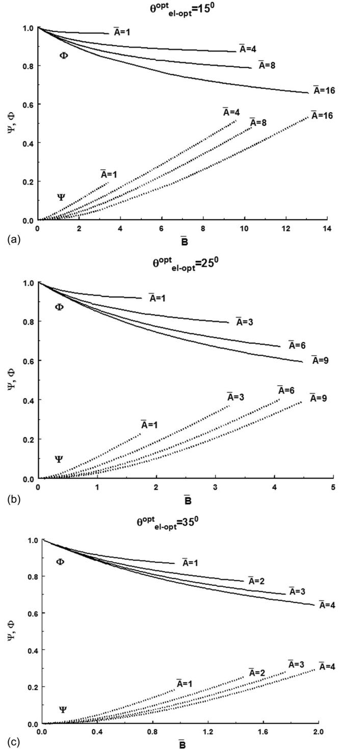
FIG. 1. Dependence of  $\Phi = [1 - 0.6\bar{A}(\theta_{opt} - \theta_{el-opt}^{opt})^2] \times [1 - \bar{B}(\sin \theta_{opt})^2]$  (solid) and  $\Psi = \Phi(\theta_{opt}) - \Phi(\theta_{el-opt}^{opt})$  (dashed) on  $\bar{B}$  for several values of the parameter  $\bar{A}$ .
