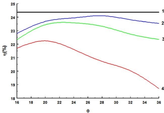
FIG. 4. Efficiency as a function of  $\theta$ . Curve 1 (black line) shows the case of no spreads; curve 2 (blue line) shows the case of  $\alpha$  spread for  $d = 3.2$  mm; curve 3 (green line) shows the case of both spreads in  $R_b$  and  $\alpha$  for  $d = 3.2$  mm; and curve 4 (red line) shows the effect of both spreads for  $d = 6.4$  mm.
