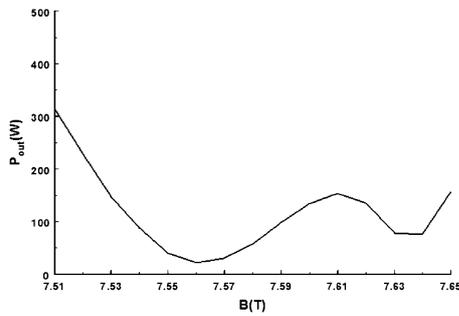
Fig. 6. Output power as a function of magnetic field. Here,  $I_{op} = 0.2$  A.
