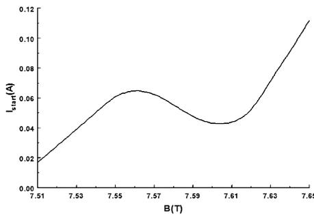
Fig. 7. Starting current as a function of magnetic field.
