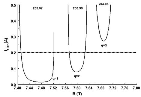
**Fig. 2.** Starting current as a function of magnetic field. The operating current  $I_{op} = 0.2$  A is marked by the horizontal dashed line. The numbers inside the starting current curves correspond to the oscillation frequencies in GHz listed in Table I.
