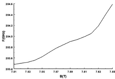
**Fig. 3.** Frequency as a function of magnetic field.
