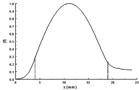
**Fig. 1.** Absolute value of the field profile of the  $TE_{0,3,1}$  mode. The middle section of the cavity is between the two vertical dashed lines.
