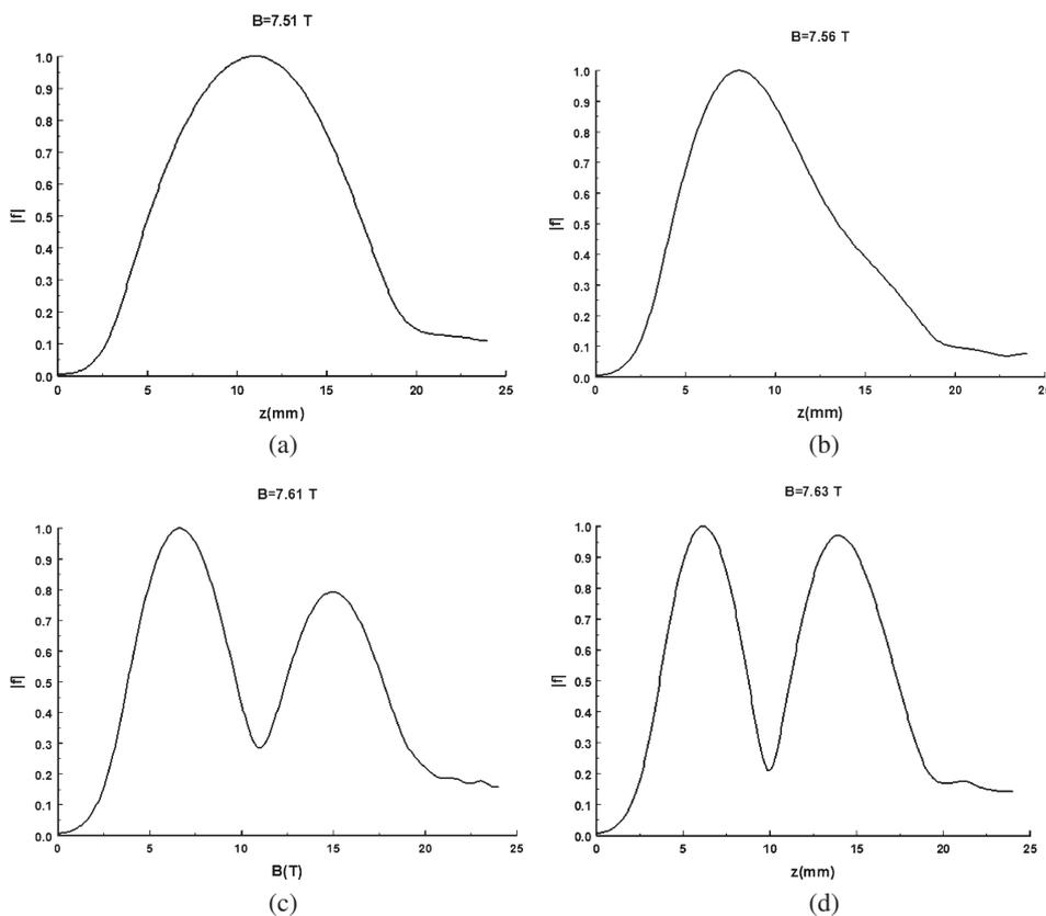
**Fig. 5.** Field profiles for selected magnetic fields. (a)  $B = 7.51$  T, (b)  $B = 7.56$  T, (c)  $B = 7.61$  T, and (d)  $B = 7.63$  T.
