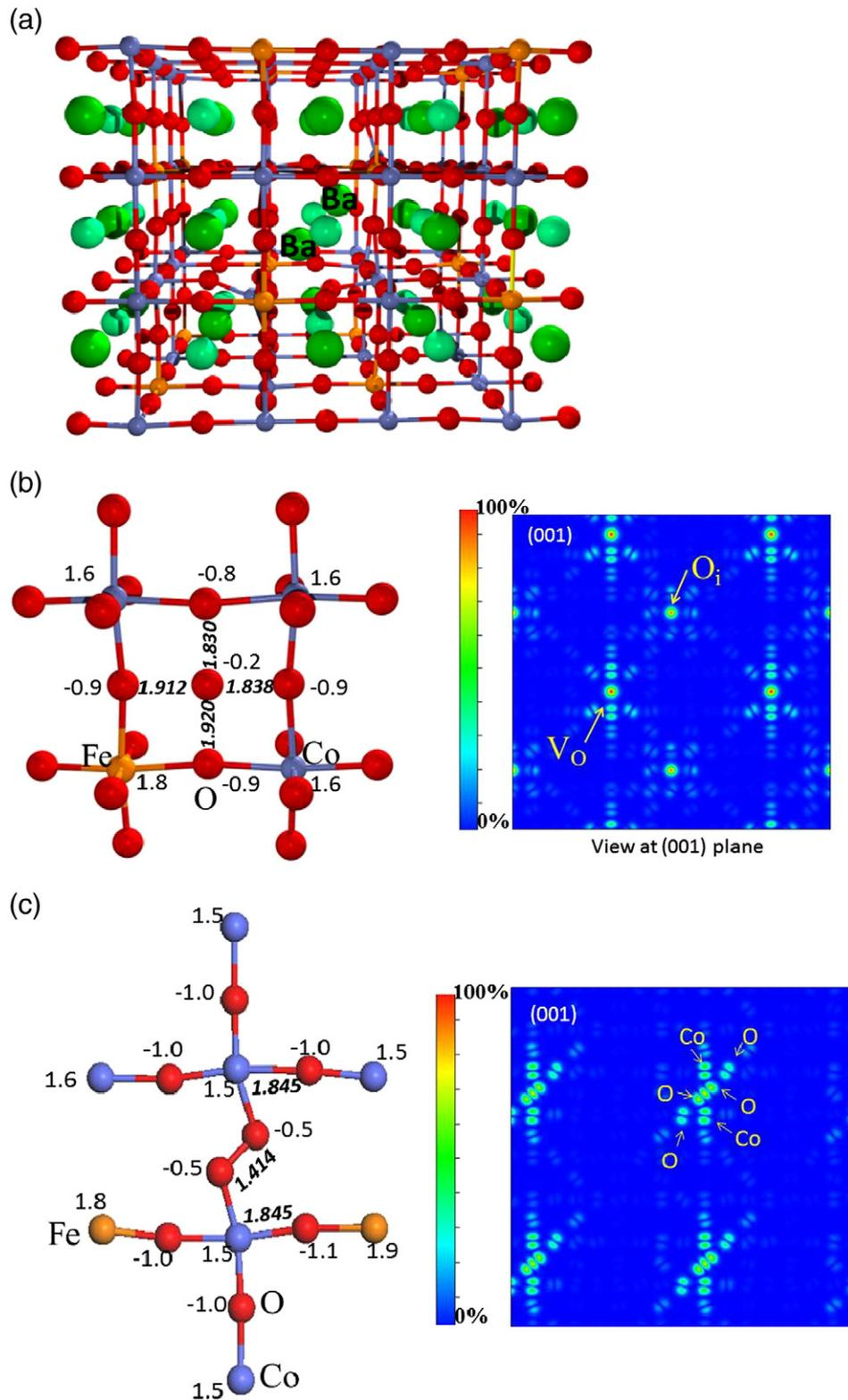
**Fig. 1.** (a) Ba–Ba split interstitial defect in the BSCF crystalline lattice and (b) details of oxygen hollow and (c) Co–O–Co oxygen split interstitial configuration, with the atomic charges, interatomic distances, and the differential electronic density map are shown.
