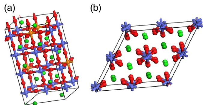
**Fig. 2.** Schematic view of the supercells of the a) cubic and b) hexagonal (2H) BSCF perovskite structures.
