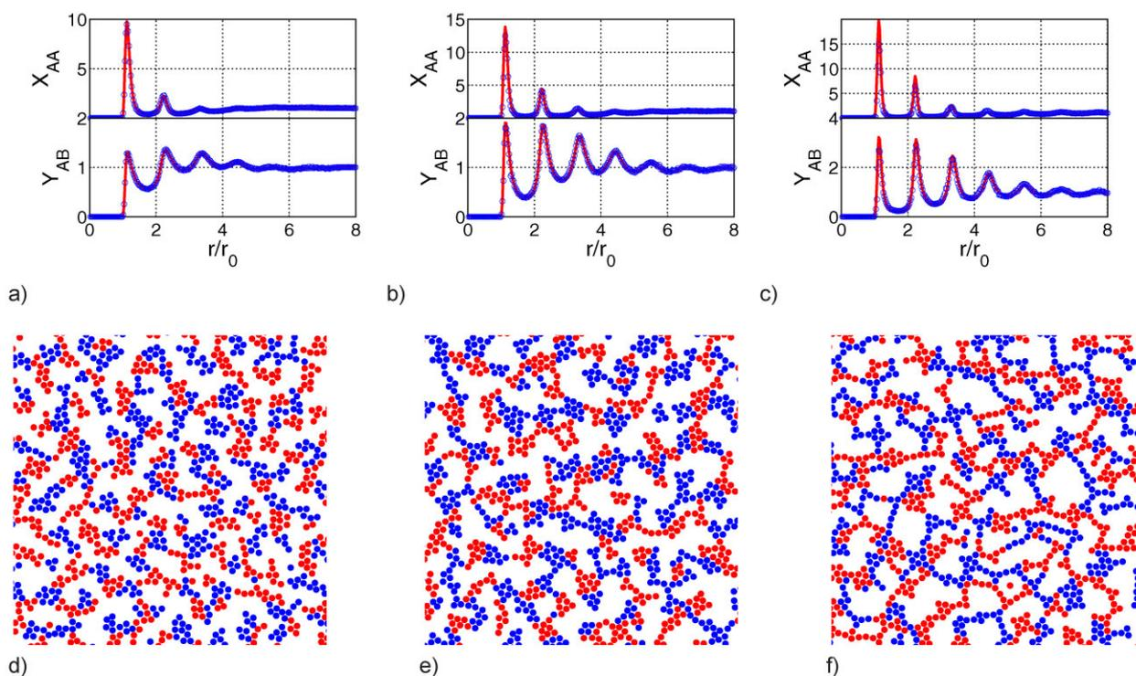
**Figure 3** Theoretical (curves) and improved RMC simulated (circles) correlation functions for 2D systems at different times (a–c) and corresponding fragments of lattice snapshots (d–f).
