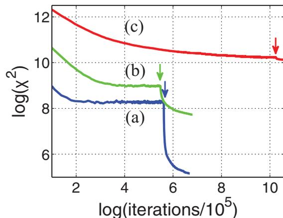
**Figure 4** Consecutive application of reversible- and irreversible improved RMC method in 2D case. Curves (a–c) reflect CF development in time and correspond to Fig. 3(a–c).
