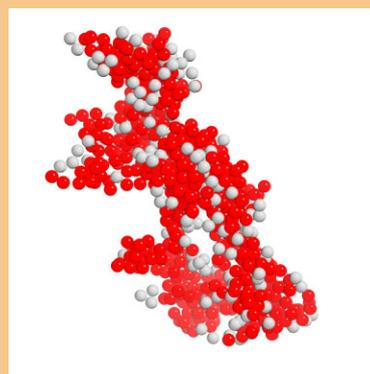
Example of 3D structure of self-assembled nanoparticles interacting via short-range LJ and long-range Coulomb potentials obtained by improved reverse Monte Carlo simulations.
