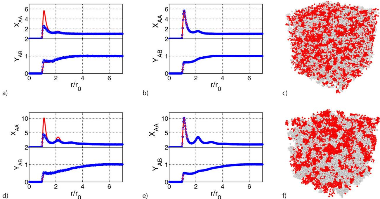
**Figure 1** Comparison of standard RMC method (a) and (d) with improved RMC (b) and (e) for 3D system. Correlation functions are marked by line and circles for theoretical and RMC results, respectively. The CF deviation from the unity means development of spatial correlations. The snapshots obtained by improved RMC are given in (c) and (f).
