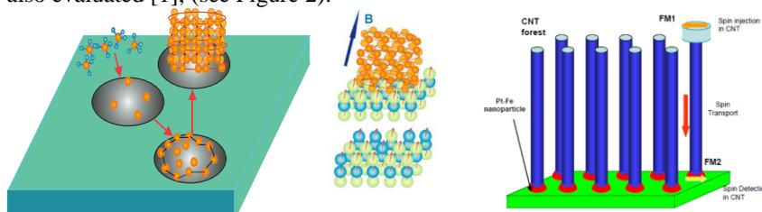
FIGURE 2 Model of CNTs growth in a magnetically controlled CVD process based on Fe-Pt nanodrops catalysts. CNTs forest is considered as a prototype of the magnetic memory, where ferromagnetic nanoparticles serve as cells of the magnetic memory.
