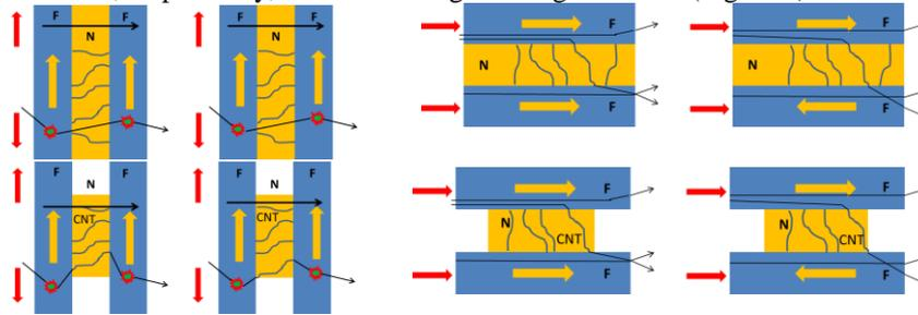
FIGURE 3a Giant magneto-resistance (GMR) device. *Current perpendicular to the plane* (CPP) spin-valve. A thin normal metal spacer (N-e.g.,CNT metal-like:) separates two ferromagnets (F).
