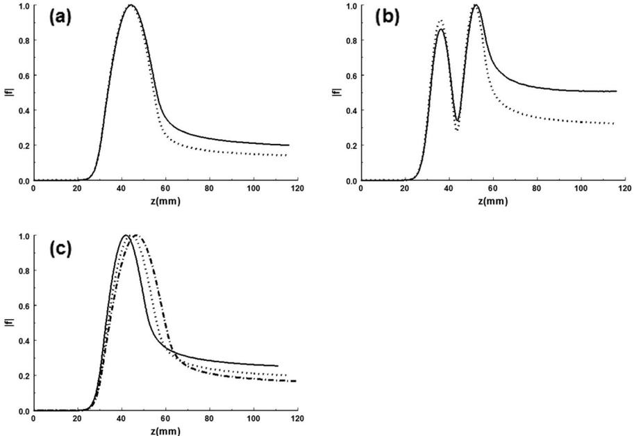
**Fig. 6** Axial structures of the modes with one and two axial variations: **a** the mode with  $q=1$ ,  $L=25$  mm, a linear up taper with two angles of tapering  $3^\circ$  (solid line) and  $1.29^\circ$  (dotted line); **b** the mode with  $q=2$  in the same resonator; **c** the mode with  $q=1$  in resonators of a different length  $L=20$  mm (solid line),  $L=25$  mm (dotted line),  $L=30$  mm (dash-dotted line) in the case of a linear uptaper with a  $1.29^\circ$  angle
