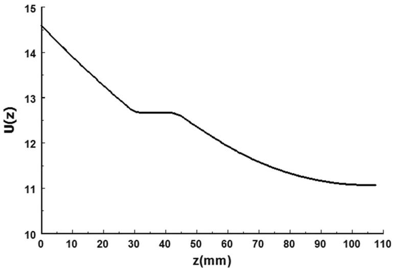
**Fig. 4** Potential well corresponding to a resonator with the original uptaper shown in Fig. 3
