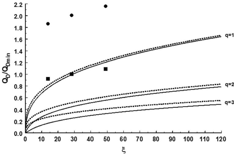
**Fig. 2** Dependencies of the ratio  $Q_D/Q_{D,\min}$  of the first three axial modes on the parameter of irregularity  $\xi$  defined by a general formula (13) (solid lines) and by an asymptotic formula (14) (dashed lines). Circles and squares show results of simulations described in Sect. 5 for  $q=1$  and  $q=2$ , respectively
