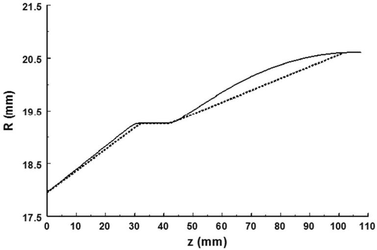
**Fig. 3** Resonator profile of the 1 MW, European gyrotron for ITER with different uptapers. The original profile of the KIT resonator is shown by a *solid line*; the linear profile discussed below is shown by the *dotted line*
