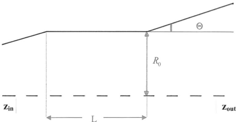
**Fig. 1** Schematic of a straight waveguide connected with the linear uptaper
