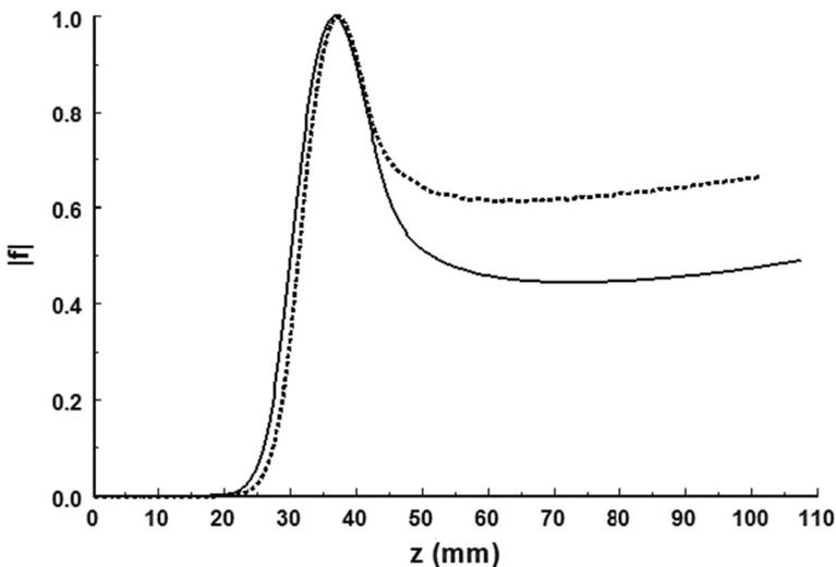
**Fig. 5** Axial profiles of the  $q=1$  mode in the original version (*solid*) of the KIT resonator and the one with the linear uptaper (*dashed*)
