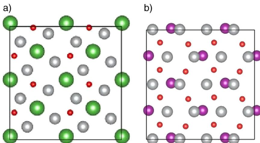
Fig. 4. Adsorption of Ag monolayer on the (001)  $\text{LaMnO}_3$  surface: a) LaO-terminated and b)  $\text{MnO}_2$ -terminated. Green, purple, red, and gray balls denote La, Mn, O, and Ag ions, respectively.
