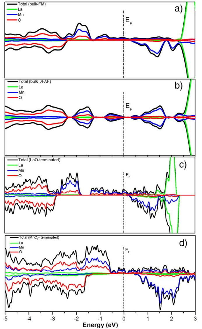
**Fig. 1.** DOS of the perfect LMO: a) perfect FM bulk, b) A-AF bulk, c) LaO-termination, and d) MnO<sub>2</sub>-termination surfaces. The Fermi energy is taken as zero.
