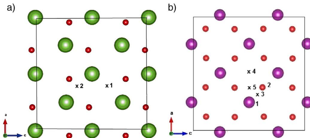
**Fig. 2.** Atomic Ag adsorption on the  $LaMnO_3$  (001) surface a) stable adsorption sites on the LaO-terminated: 1—“hollow-1” position and 2—“hollow-2” position. b) Stable adsorption sites on the  $MnO_2$ -terminated: 1—atop Mn, 2—atop O, 3—“bridge Mn–O” position, 4—“hollow” position, and 5—“bridge O–O” position. Green, purple, and red balls denote La, Mn, and O ions, respectively.
