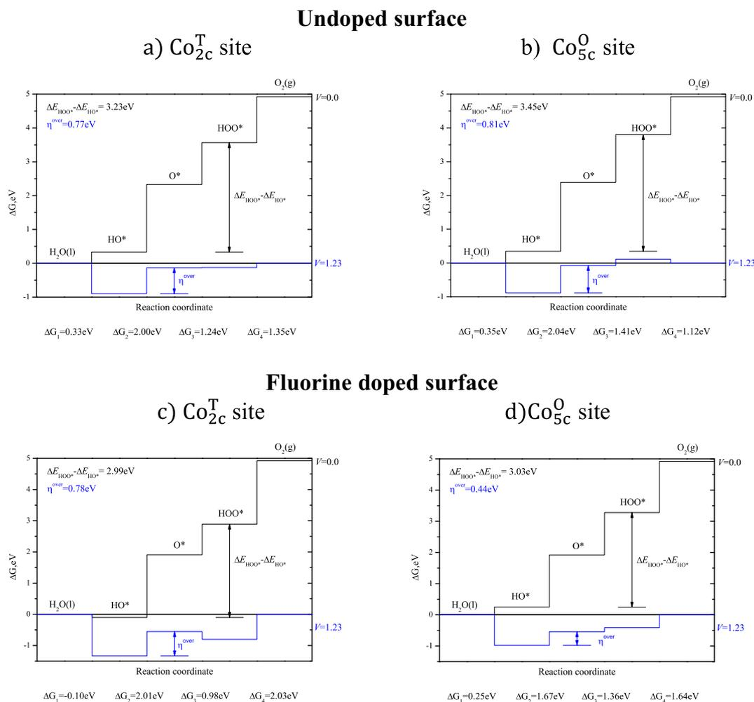
**Fig. 6.** Free-energy diagram at pH = 0 and T = 298 K for the four steps of the OER at V = 0 and V = 1.23 V. Results for the  $\text{Co}_{2c}^T$  and  $\text{Co}_{5c}^O$  sites at 0.2 ML water coverage for undoped and F-doped surfaces shown; For each case the characteristic difference  $\Delta E_{\text{OOH}^*} - \Delta E_{\text{HO}^*}$  [4,13] and  $\eta^{\text{over}}$  are shown.
