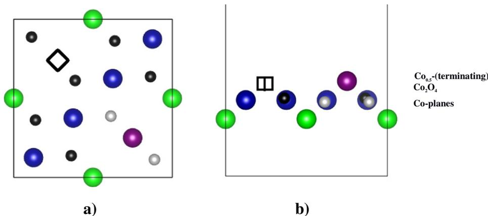
Fig. 2.  $\text{Co}_3\text{O}_4$  (100)  $\text{Co}_{0.5}$ -terminated surface top view (a) and side view (b). Color coding:  $\text{Co}_{5c}^{\text{O}}$ , blue;  $\text{Co}_{4c}^{\text{T}}$ , green;  $\text{Co}_{2c}^{\text{T}}$ , purple;  $\text{O}_{3c}$ , black;  $\text{O}_{4c}$ , gray; The empty cube indicates Co site.
