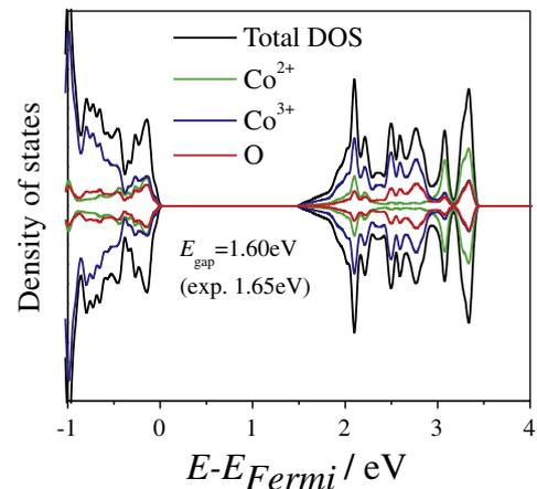
**Fig. 1.** The electronic DOS of a pure  $\text{Co}_3\text{O}_4$ .
