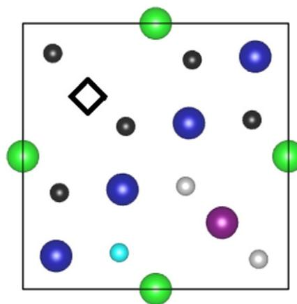
Fig. 3. Top view and side view of fluorine doping on the  $\text{Co}_3\text{O}_4$  (100)  $\text{Co}_{0.5}$ -terminated surface. Color coding:  $\text{Co}_{5c}^{\text{O}}$ , blue;  $\text{Co}_{4c}^{\text{T}}$ , green;  $\text{Co}_{2c}^{\text{T}}$ , purple;  $\text{O}_{3c}$ , black;  $\text{O}_{4c}$ , gray; F, cyan. The empty cube indicates Co site.
