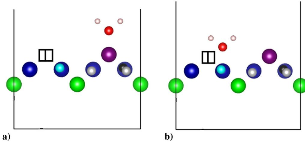
**Fig. 4.** Side view of H<sub>2</sub>O adsorption at the Co<sub>2c</sub><sup>T</sup> (a) and Co<sub>5c</sub><sup>O</sup> (b) sites on the Co<sub>3</sub>O<sub>4</sub> (100) Co<sub>0.5</sub>-terminated surface. Color coding: Co<sub>5c</sub><sup>O</sup>, blue; Co<sub>4c</sub><sup>T</sup>, green; Co<sub>2c</sub><sup>T</sup>, purple; O<sub>3c</sub>, black; O<sub>4c</sub>, gray; F, cyan; O<sub>ads</sub> (H<sub>2</sub>O), red; H, white. The empty cube indicates Co site.
