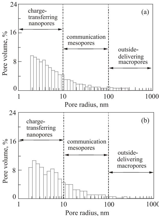
Fig. 2. Pore size distributions of  $\text{Cu}_{0.4}\text{Co}_{0.4}\text{Ni}_{0.4}\text{Mn}_{1.8}\text{O}_4$ -macro (a) and  $\text{Cu}_{0.4}\text{Co}_{0.4}\text{Ni}_{0.4}\text{Mn}_{1.8}\text{O}_4$ -micro (b) modified ceramics.
