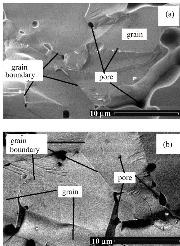
Fig. 1. Scanning electron micrographs of fracture section of  $\text{Cu}_{0.4}\text{Co}_{0.4}\text{Ni}_{0.4}\text{Mn}_{1.8}\text{O}_4$ -macro (a) and  $\text{Cu}_{0.4}\text{Co}_{0.4}\text{Ni}_{0.4}\text{Mn}_{1.8}\text{O}_4$ -micro (b) modified ceramics.
