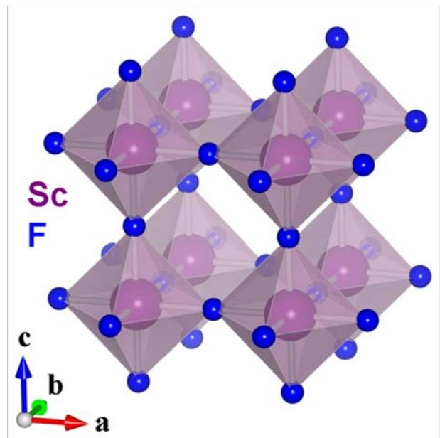
Fig. 1. Schematic view of cubic  $\text{ScF}_3$  structure (space group  $Pm-3m$  (221)) built up of  $\text{ScF}_6$  regular octahedra joined by corners (small balls are fluorine atoms, large balls are scandium atoms). All Sc–F–Sc angles are equal to  $180^\circ$ .
