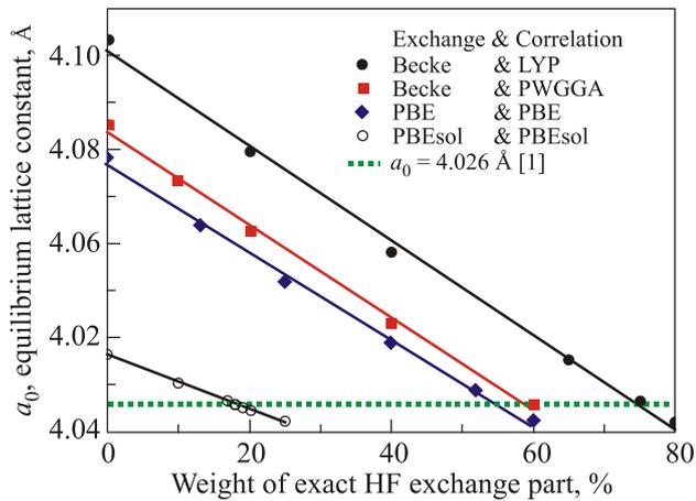
Fig. 2. (Color online) Dependence of the equilibrium lattice constant on the weight of exact HF non-local exchange in hybrid density calculation by the LCAO method.
