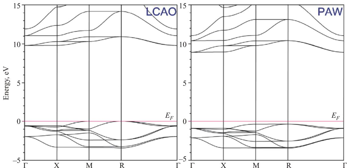
Fig. 5. The energy bands of  $\text{ScF}_3$  crystal constructed for LCAO calculations with PBEsol & PBEsol functional and weight of exact HF nonlocal exchange  $w_{\text{HF}} = 18\%$  (full-electron basis set, left panel) and PAW calculation with PW91 functional and  $w_{\text{HF}} = 25\%$  (LC-ECP, right panel). The energies are given in eV, Fermi level  $E_F$  is shown with horizontal magenta line.
