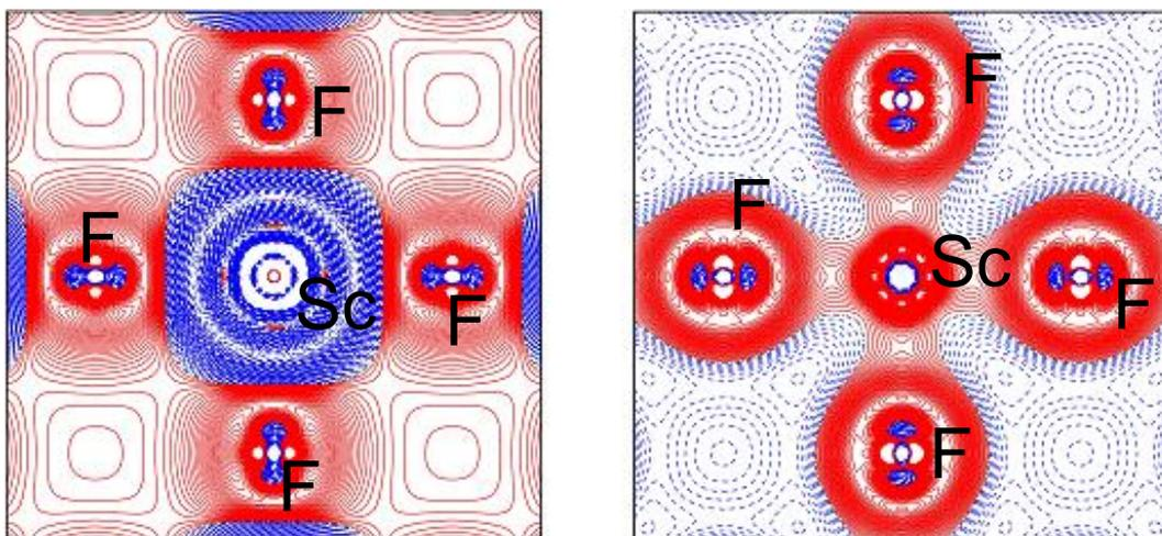
Fig. 3. (Color online) Plots of the charge density difference in (100) plane of  $\text{ScF}_3$  between the full charge density of the crystal and electronic density of non-interacting atoms (left panel) and ions (right panel) obtained using “PBEsol & PBEsol” functional with  $w\text{HF} = 18\%$ . Solid (red) and dashed (blue) isolines correspond to positive (excess) and negative (deficiency) electron density difference, respectively.
