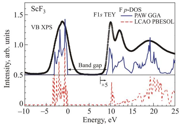
Fig. 4. (Color online) A comparison of the F  $p$  density of states (DOS) calculated by means of the LCAO (dashed line) and PAW (solid line) methods with valence-band photoelectron [37] and F  $1s$  x-ray absorption spectra [5]. The amplitude of the DOS in the conduction band was multiplied by a factor of 5. Energy scale is given with respect to the calculated top of the valence band. Experimental spectra have been aligned to match best the calculations.
