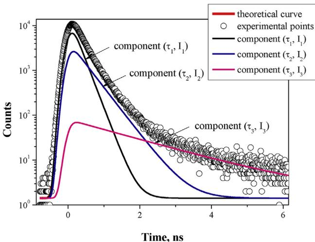
Fig. 3. Typical PAL spectrum for  $\text{Ge-Ga-S-CsCl}$  glasses decomposed into three combined positron-positronium components.
