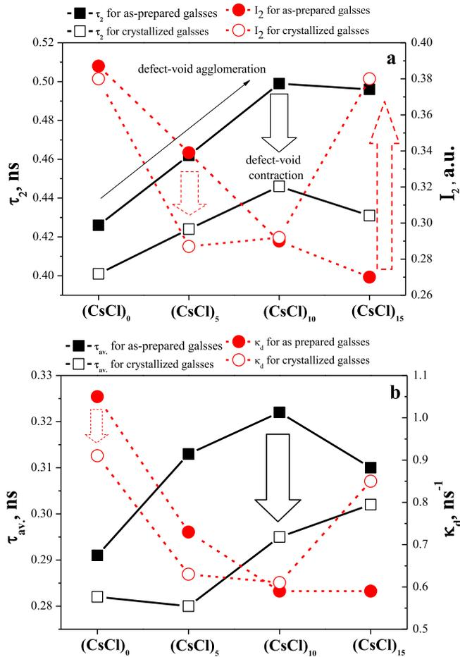
Fig. 4. Defect-related ( $\tau_2$ ,  $I_2$ ) component (a) and average lifetime  $\tau_{av}$  and positron trapping rate  $\kappa_d$  in defects (b) for as-prepared and crystallized GeSe<sub>2</sub>–Ga<sub>2</sub>S<sub>3</sub>–CsCl glasses as function of CsCl content.
