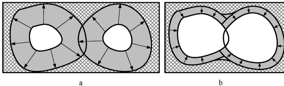
Fig. 5. Schematic illustration of free-volume void agglomeration due to modification of Ge–Ga–S glassy matrix by CsCl addition (a) and void constriction (b) caused by full crystallization process.
