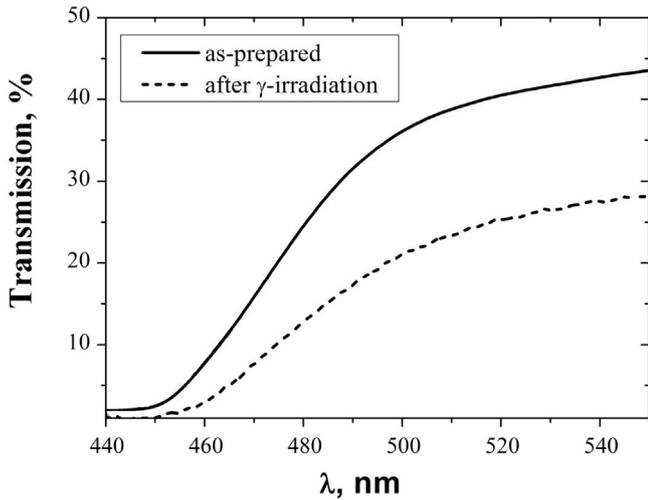
Fig. 2. Transmission spectra for as-prepared and  $\gamma$ -irradiated  $80\text{GeS}_2\text{-}20\text{Ga}_2\text{S}_3$  base glasses.
