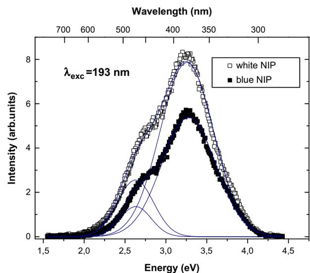
Fig. 4. Photoluminescence spectra of White and Blue NIP's under UV-light excitation ( $\lambda = 193$  nm) and their Gaussian deconvolution.
