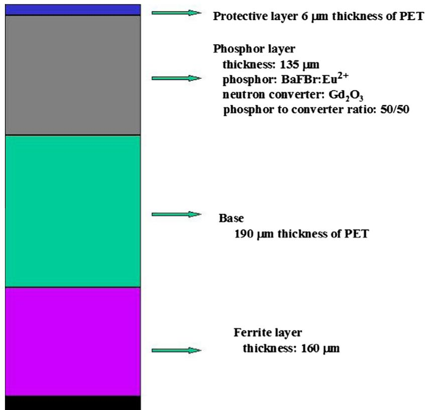
Fig. 1. Structure of the Fuji BAS-ND image plate.
