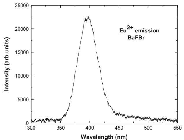
Fig. 2. Spontaneous luminescence spectrum of the White NIP under X-ray excitation.
