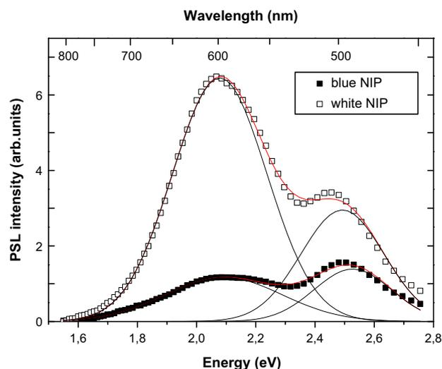
Fig. 3. Stimulation spectra of X-ray irradiated Blue and White NIP's and their Gaussian deconvolution. The stimulation spectra were observed by measuring the PSL emission of  $\text{Eu}^{2+}$  at about 400 nm.
