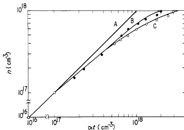
Figure 1. The simulated production curves: A, absence of recombination; B,  $\alpha = 10^{19} \text{ s}^{-1} \text{ cm}^{-3}$ ; C,  $\alpha = 10^{16} \text{ s}^{-1} \text{ cm}^{-3}$ . The divergence between the straight line A and the F, H centre accumulation curve yields the concentration of both tunneling products ( $F^+$ , I centres) and aggregate ( $F_2$ ,  $H_2$ , ...) centres.
