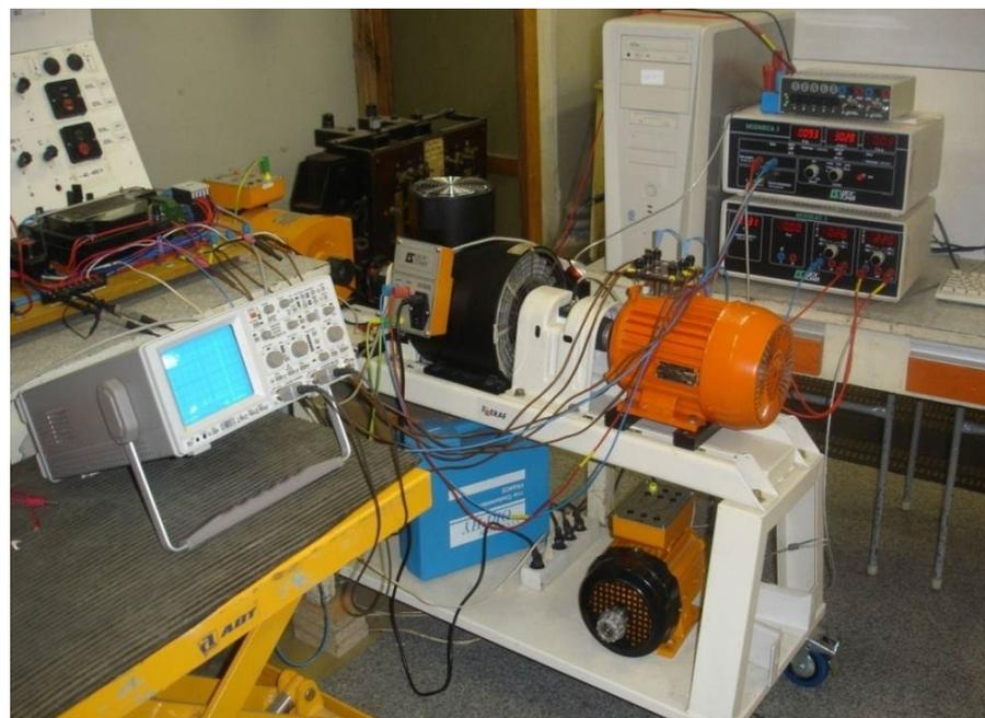
**Figure 10.** Setup of the induction motor for measuring starting characteristics.
