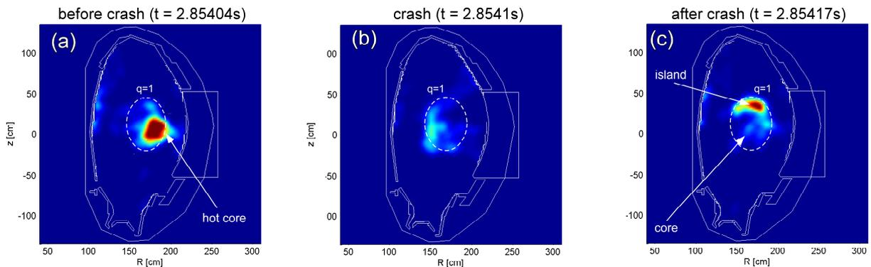
**Fig.6.** Soft X-ray tomography of the sawtooth crash (#25854,  $t=2.85s$ ). Three different time frames are shown: (a) hot core rotates in clockwise direction before the crash; (b) crash phase; (c) hot island rotates in clockwise direction after the crash.  $q=1$  position is marked by the dashed line. (Each figure has its own color scheme to increase the contrast.)
