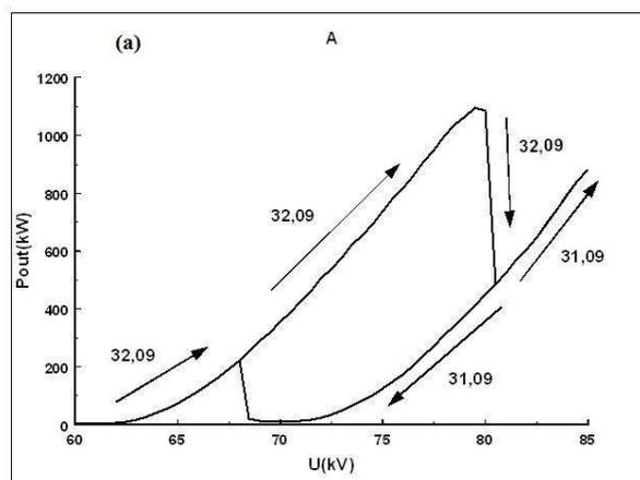
**Fig. 5.** Output power as a function of voltage in a gyrotron with the cavity A. Calculations were carried out from  $60\text{kV}$  to  $85\text{kV}$  and from  $85\text{kV}$  to  $60\text{kV}$ . The parasitic  $TE_{31,09}$
