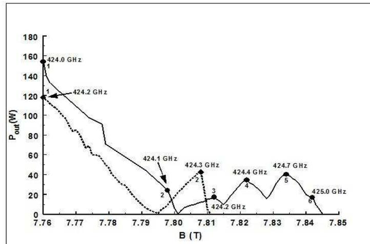
**Fig. 7.** Output power and frequency as a function of the magnetic field in the cylindrical cavity (dashed) and in the uptapered cavity (solid). Positions of the axial wave numbers  $q$  are marked by diamonds and dots respectively. The output power forms a fingerlike shape. In the mode transition region, the output power is small but nonzero and the oscillation frequency can be smoothly tuned.
